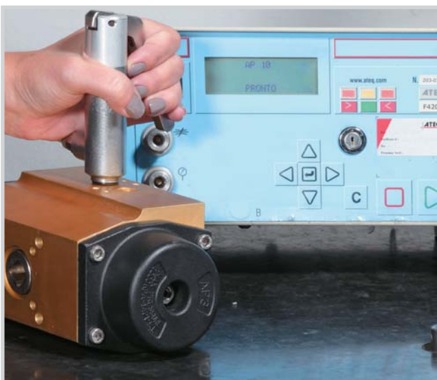
Leack test machine. For pneumatic rotary actuators.
