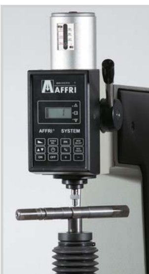
Hardness testing machine. Metal and rubber materials.
